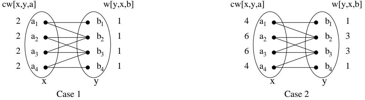
Figure 2: Weights of the values: in Case 1 the weight associated with each b_i is 1 and in Case 2 the weight associated with each b_i is its own support count with respect to x . The cumulative weight of each a_i \in D(x) is computed for each case accordingly.
